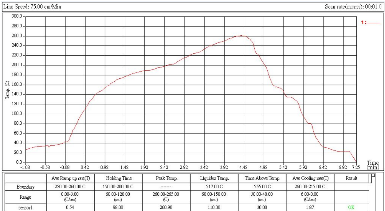
Figure 8.3 Solder Reflow Profile
